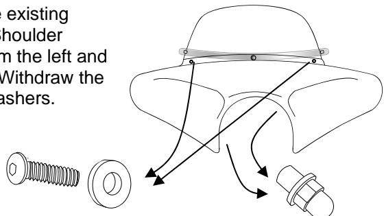
5. Align the Polished Slotted Stainless Steel Trim, Slim Style over the left and right holes and insert Stainless Steel Button Head Screws. Secure in place with Acorn Nut Shoulder
